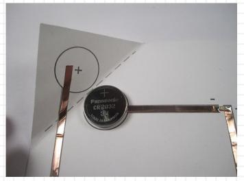
HOW TO MAKE A SIMPLE SWITCH BY FOLDING A CORNER OF YOUR PAPER TO CLOSE THE CIRCUIT
